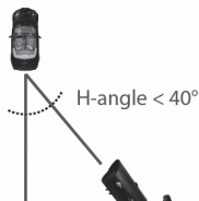
H-angle less than 40° correct
