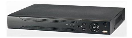
Up to 8 cameras with 1080p realtime preview H.264 dual-stream video compression All channel 2CIF or 2ch D1 & 6ch CIF HDMI / VGA simultaneous video output All channel synchronous realtime playback, GRID interface & smart search Support 1 SATA HDDs up to 4TB, 2 USB2.0 Multiple network monitoring: Web viewer, CMS(DSS/PSS) & DMSS
