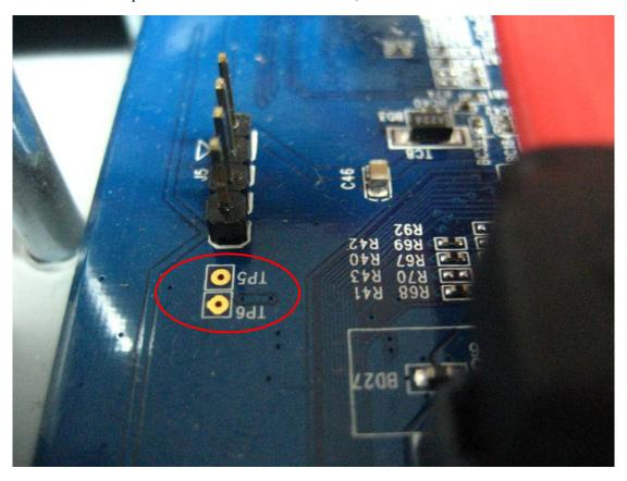
STEP3: Disconnect the DVR power. Then, make the chip resistor short-circuited with a conductive object (such as forceps) as indicated below, and re-connect the power. Remove the conductive object when you hear a short beep sound, and wait till the DVR reboots.
