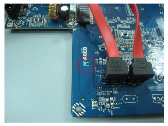
STEP3 : Disconnect the DVR power. Then, make the chip resistor short-circuited with a conductive object (such as forceps) as indicated below, and re-connect the power.Remove the conductive object when you hear a short beep sound, and wait till the DVR reboots.
