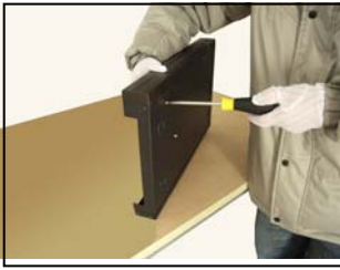
④ fix the screw of hard disk
