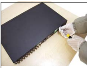
① disassemble the screw
