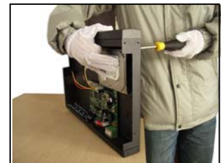
③ fix the screw of hard disk
